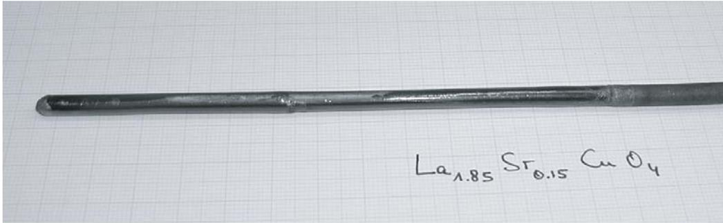
**Figure 2:** Single crystal of  $\text{La}_{2-x}\text{Sr}_x\text{CuO}_4$  grown in the mirror furnace at WMI. The last about 6 cm on the left end of the sample are formed by a single crystallite.
